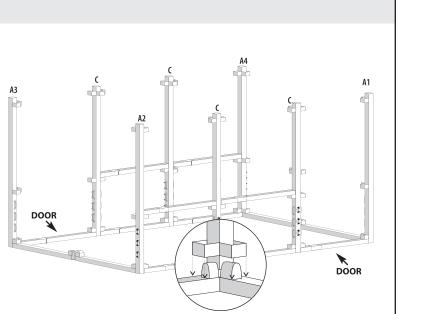
Place the middle **B** crossbars into the middle fittings of the **A** bars. Then place the top crossbars directly above them. Use the mallet to tap fittings together. NOTE: The door area does not get a middle crossbar.
