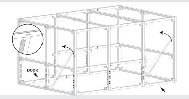
Each Sukkah has 3 mehadrin bands (2 sets) which go around 3 walls of the Sukkah. The door wall remains open. Starting with the A1 upright to the right of the door, hook a band into the top loop (diagram 1), and continue counter clockwise around the Sukkah. Thread the bands through the guides on each upright, (diagram 2) ending with the back D upright. Fasten the band properly.\*
