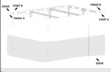
Place bamboo sticks (not included) over the top crossbars using the brass clips. The bamboo sticks should be evenly spaced from each other and from the walls of the Sukkah.
