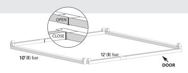
While facing the longer (door) side of the Sukkah looking in, Start with the corner on your right. Insert the **A1** upright bar onto the crossbar pins.
