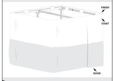
Place bamboo sticks (not included) over the top crossbars using the brass clips. The bamboo sticks should be evenly spaced from each other and from the walls of the Sukkah.
