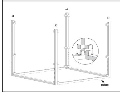
Place the middle **B** crossbars into the middle fittings of the **A** & **C** bars. Then place the top crossbars directly above them. Use the mallet to tap fittings together.
