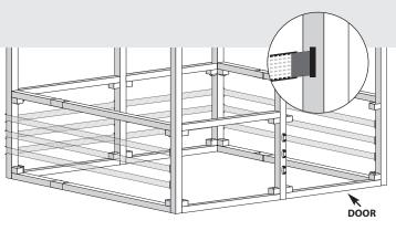
Open the nylon and find the end with the door on it. The side with the screen faces the inside. The lighter color goes on top.
