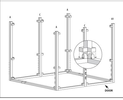
Place the middle **B** crossbars into the middle fittings of the **A** & **C** bars. Then place the top crossbars directly above them. Use the mallet to tap fittings together.
