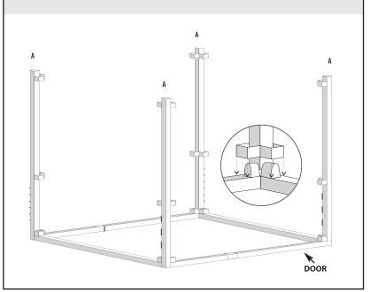
Place the middle **B** crossbars into the middle fittings of the **A** bars. Then place the top crossbars directly above them. Use the mallet to tap fittings together. NOTE: The door side does not get a middle crossbar.
