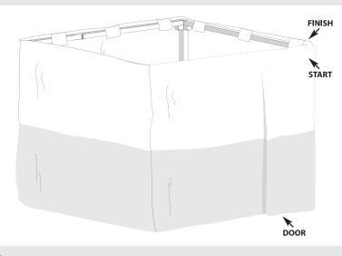
Place bamboo sticks (not included) over the top crossbars using the bamboo holders. The bamboo sticks should be evenly spaced from each other and from the walls of the Sukkah.
