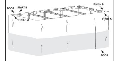
Use brass extensions to create wood\* crossbeams (2"x3", not included), enough to cover 12'6" span. Place over the top crossbars.
