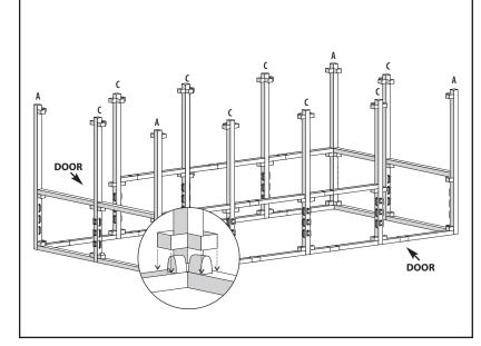
Place the middle **B** crossbars into the middle fittings of the **A** & **C** bars. Then place the top crossbars directly above them. Use the mallet to tap fittings together.
