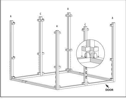
Place the middle **B** crossbars into the middle fittings of the **A** & **C** bars. Then place the top crossbars directly above them. Use the mallet to tap fittings together. NOTE: The door area does not get a middle crossbar.
