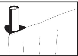
Continue round the Sukkah till reaching the door. Adjust the door fitting (H) to the correct position for the door and tighten, then place last grommet over pole. Attach the door hooks over pole then attach the hooks to the canvas through the small grommets then close the hooks.
