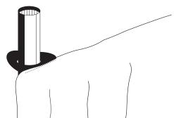
Continue round the Sukkah till reaching the door. Adjust the door fitting (H) to the correct position for the door and tighten, then place last grommet over pole. Attach the door hooks over pole then attach the hooks to the canvas through the small grommets then close the hooks.
