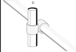
First insert the (A) poles into fittings and tighten, then insert the (B) poles into fittings, and tighten.
