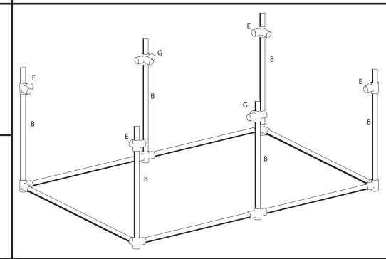
Attach top fitting about 1 ½ inch down on the pole (fittings can be moved up or down to tighten or loosen canvas), and then tighten screw until tight.
