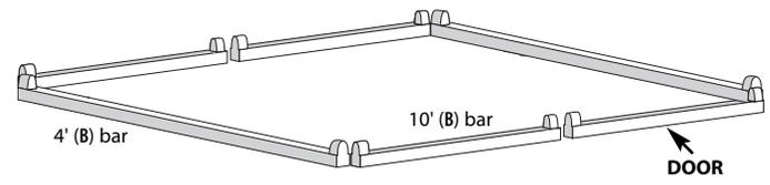
**2** While facing the longer (door) side of the Sukkah looking in, Start with the corner on your right. Insert the **A1** upright bar onto the crossbar pins. (make sure the arrow is facing up, and the closed loops, are facing the back of the Sukkah.)
