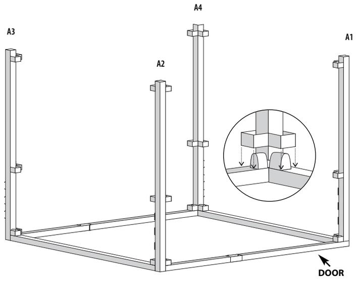
**3** Place the middle **B** crossbars into the middle fittings of the **A** bars. Then place the top crossbars directly above them. Use the mallet to tap fittings together.
