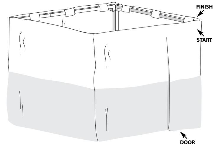
**6** Place wood\* crossbeams (1"x2", not included) over the top crossbars using the brass clips. The wood beams should be evenly spaced from each other and from the walls of the Sukkah.
