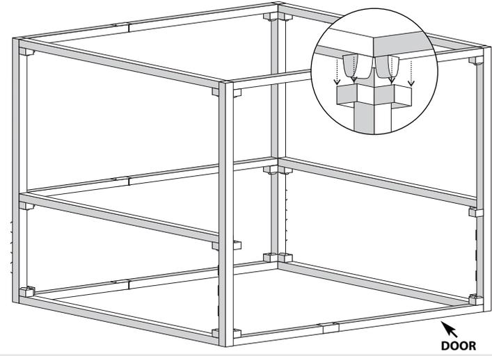
**4** Each Sukkah has 3 mehadrin bands which go around three walls of the Sukkah. The door wall remains open. Starting with the upright to the right of the door **A1**, hook a band into the top loop (diagram 1), and continue counter clockwise around the Sukkah. Thread the band through the guides on each upright, (diagram 2) ending with the **A2** corner to the left of the door.
